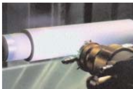
Plasma spraying of a shaft
