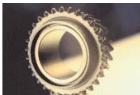
Laser beam welding of a gear for automotive manual shifter, 16MnCr5 hardened
