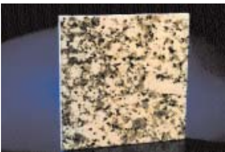
Anti-slip preparation of polished flooring with laser micro structuring
