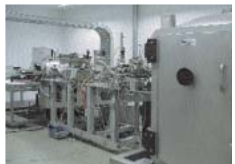
Overall view of the EUV reflectometer
