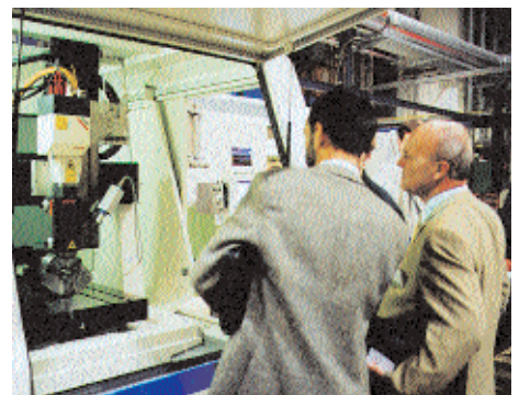
Demonstration of a hardening machine with an integrated high power diode laser in the laser hall of IWS
