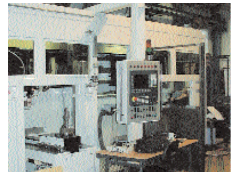
Laser induction-welding system in batch manufacturing at Getrag Ford Transmissions Cologne
