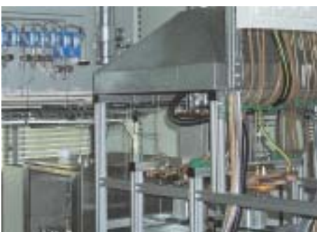
Arc-jet CVD reactor during the coating of stainless steel
